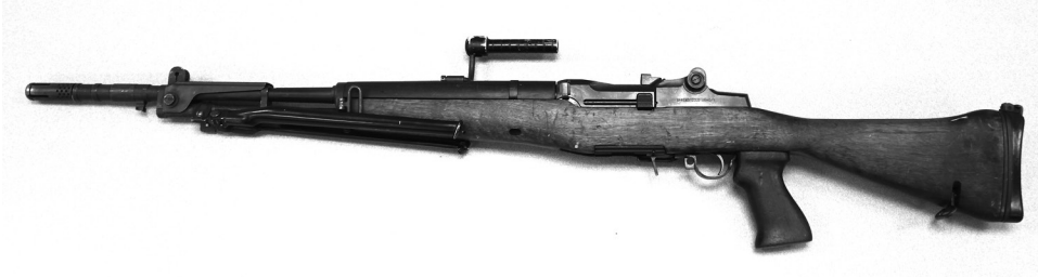
Figure 4.57 (See color insert.) The M14-pattern rifle manufactured by Beretta as the BM59. There are definite similarities, but note the distinct differences between the M14 and the BM59. This example has a bipod, a grenade-launcher spigot on the muzzle, a grenade-launching ladder-type sight, and a pistol grip instead of a standard rifle stock. (Image from author's collection.)
